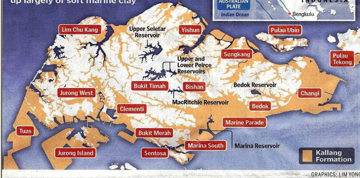
A generalized geological map of Singapore showing the occurrence of the Kallang Formation (prepared by Singapore Straits Times, 2010)
