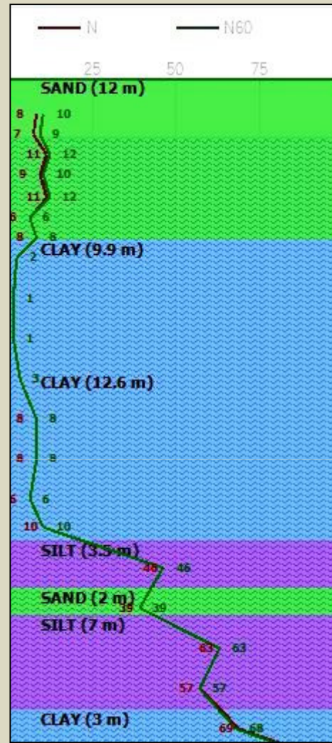
Generalized soil profiles in a reclaimed area south of Singapore.
