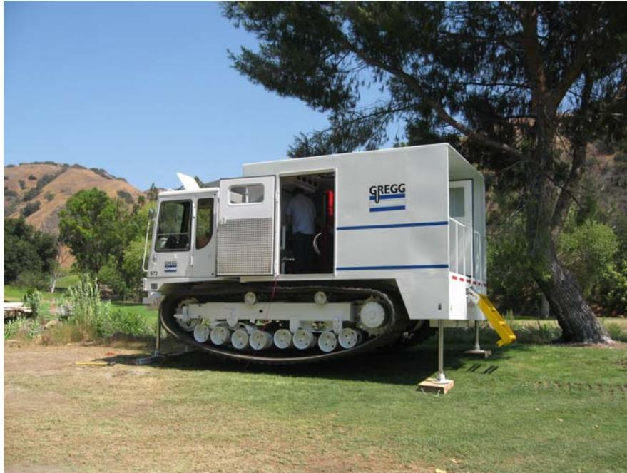
**Figure 11** Track mounted 20 ton CPT unit
