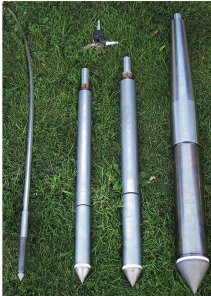
**Figure 8** Range of CPT probes (from left: 2 cm<sup>2</sup>, 10 cm<sup>2</sup>, 15 cm<sup>2</sup>, 40 cm<sup>2</sup>)
