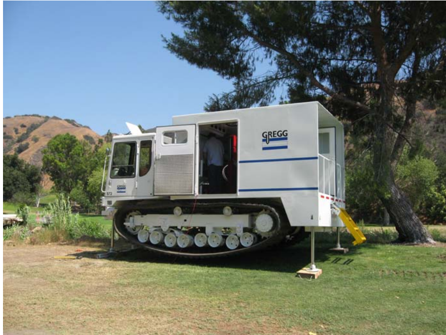
Figure 11 Track mounted 20 ton CPT unit
