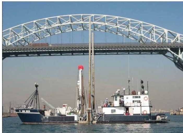
Figure 16 Quinn Delta ship with spuds
