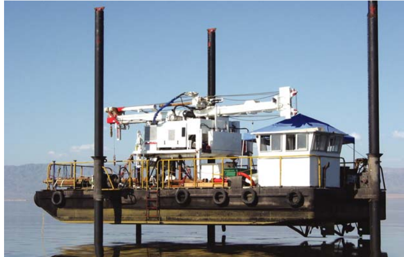
Figure 15 Mid-size jack-up boat
